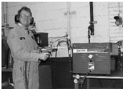
Operator John Cooper adjusts a Diamond Jet HVOF spray gun fueled by a G-TEC Natural Gas Torch Booster
