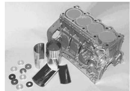
Fig. 8 Coating development includes coating of tribo-samples, single bushes, and complete light metal engine blocks
